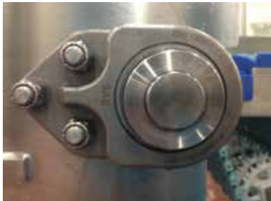
Choice Ball Machined SS on drive roller
