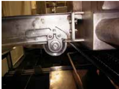
Classic Ball Machined SS with solid lube on oven input
