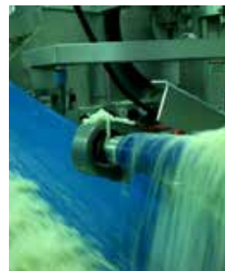
Classic Ball Machined SS with solid lube over cheese shredding
