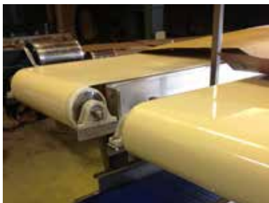
Value Ball Polymer on flat belt drum
