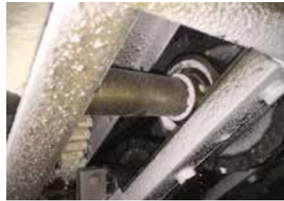
Classic Ball Stainless with solid lube in freezer
